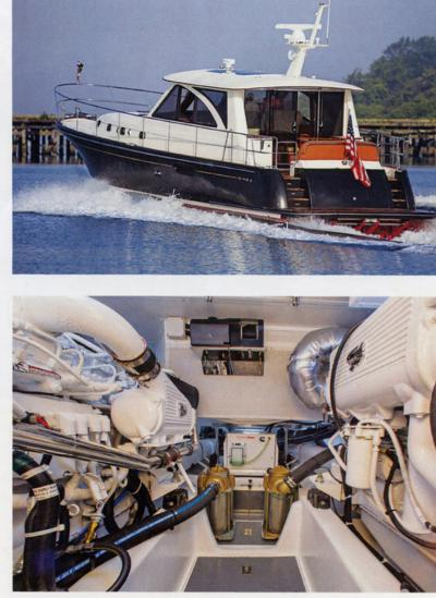
LOA: 45'10" BEAM: 14'6" DRAFT: 4'0" (props) DISPL.: 35,000 lb. (half load) FUEL: 450 gal. WATER: 120 gal. DEADRISE: 20 degrees ENGINES (tested): 2 x 593 hp Cummins QSC8.3 600 diesels w/ ZF pod drives ENGINES (std.): 2 x 450 hp Caterpillar C7 ACERT diesels BASE PRICE: \$1.350.00
